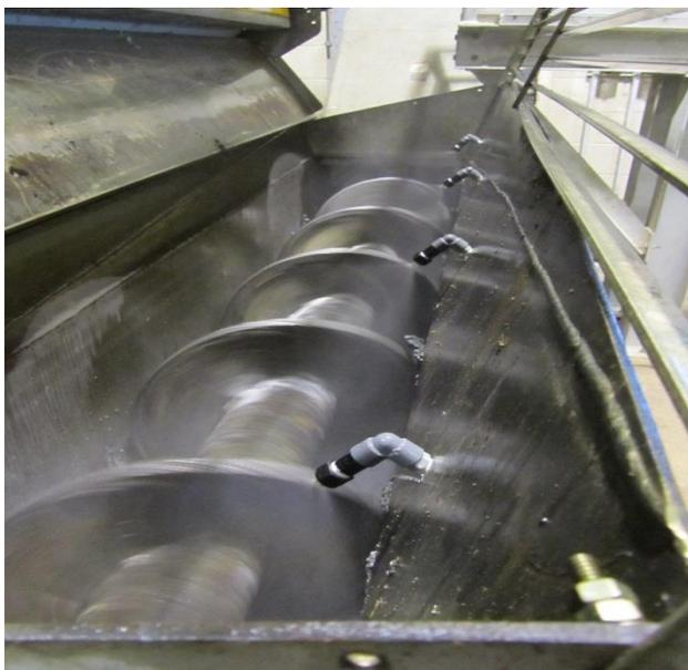
QuikSoil® 2900 is applied as the biosolids exit the belt press or centrifuge, or as they are loaded for transport. The application location should be the point which allows the maximum biosolids surface area to be contacted by the QuikSoil® 2900 and water mix.
